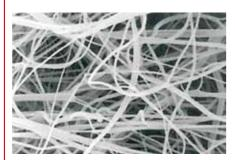
Star-pleated or cylindrical disposable filter elements made of glass fibre or melt-blown polyester or polypropylene. The highly porous filter layer provides a filtration performance of up to 99.99 % with high solids absorption and low pressure loss.
