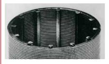
Slotted tubes consist of a profile wire that is helically coiled about a support profile and welded. The filtration rating is obtained from the distance of the coil loops. Thanks to their extremely rugged design, slotted tubes can be cleaned as often as desired. Material: 1.4435
