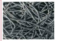
Chemicron® is a renewable metal fibre depth filter medium whose threedimensional structure gives it a high contaminant-absorption capacity and excellent retention properties. Optimal media resistance and temperature resistance up to 400 °C thanks to austenitic material 1.4404.
