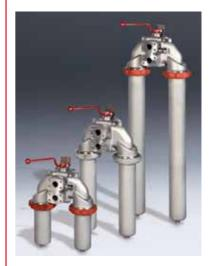
For continuous operation up to 100 bar operating pressure, the reversible variant is suitable, which consists of two filter housings with ball-valve switching. Otherwise this version corresponds to the PFL / PFM / PFH series. If desired, both side parts can be monitored by a central clogging indicator.
