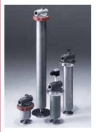
Universal filter made of stainless steel for pressures up to 100 bar, temperatures up to 200 °C and flow rates up to 120 l/min. Connection size: Cylindrical pipe thread G 1". Great variety of applications thanks to numerous sizes. Filter materials: slotted tube, wire mesh, Chemicron<sup>®</sup> metal fibre, coiled plastic candles. Special feature: no tools are required for element dismantling.
