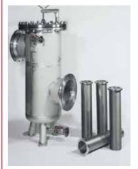
Screen basket filters are used mainly as coarse filters or pre-filters. Unlike the inline filters PRFL and PRFLD, the direction of flow is from the inside to the outside. The separated solids remain behind in the stainless steel strainer and can be removed easily and quickly. Nominal widths of DN 50 and larger are available. Materials: carbon steel or stainless steel 1.4571.
